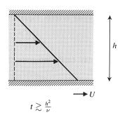
For times greater than  $\frac{h^2}{\nu}$  the flow has almost reached its steady state and the vorticity is almost distributed uniformly throughout the fluid.
